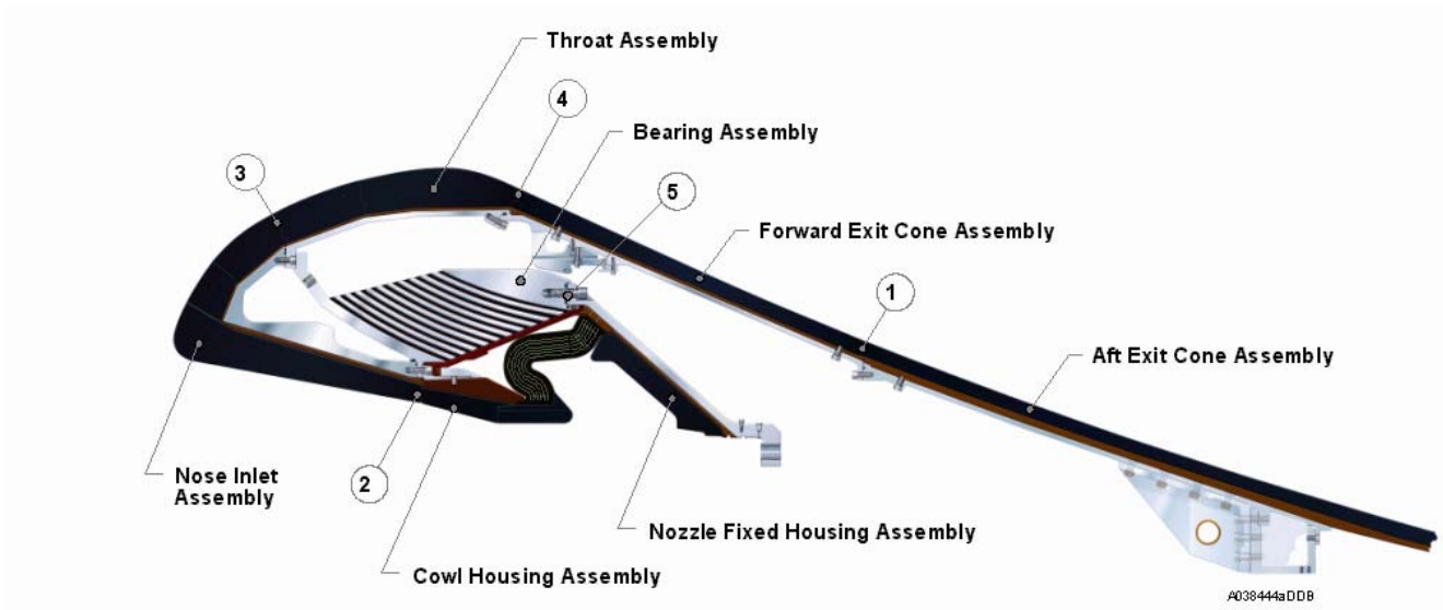
Figure 9-8. SRM Nozzle Showing Five Joints
